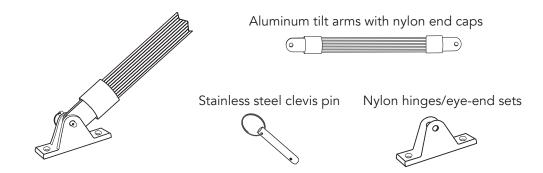
Attach a nylon hinge/eye to each stile approximately 2" from the bottom, with the screw holes 3/4" inward from the outside edge. After mounting the hinge/eyes to the shutter, allow the shutter to hang from the top mounted hinge. Position a second hinge/eye on the wall so both hinge/eyes can be pinned together when the shutter is in the closed position. Mark the location and attach the hinge/eye to the building. Repeat this procedure for the other stile.
